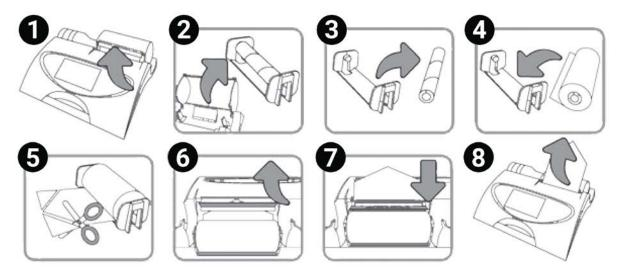
Figure 4 – Fitting a new paper roll.
