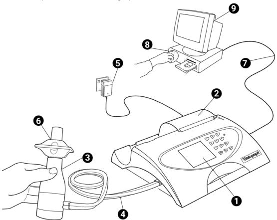
Figure 1 Main components of ALPHA
